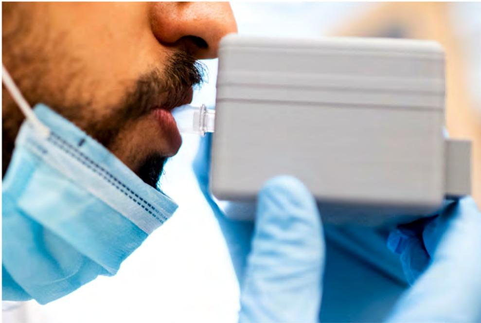
The breathalyzer designed by Nian Sun's lab uses electrochemical sensors made to catch viral particles from the air, including from exhaled breath. PHOTOGRAPH: RUBY WALLAU/NORTHEASTERN UNIVERSITY
